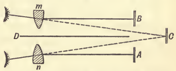
FIG. 257. — Illustrating the Principle of the Stereoscope.
